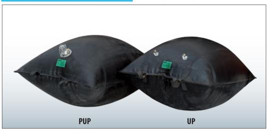
These pillow shaped pipe stoppers are mainly used in sanitary sewers and storm sewers. Their advantage is in their ability to be inserted into the pipe through standard 24" manholes. The special Kevlar reinforcement enables us to manufacture these stoppers in large diameters. The standard product line fits pipes from 40" to 88" inches in diameter.
