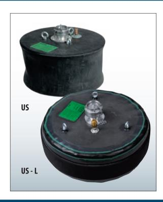
These short, light and easy-to-handle stoppers are used for leak tests of standard gullies using water or air as the testing medium according to DIN EN 1610.
